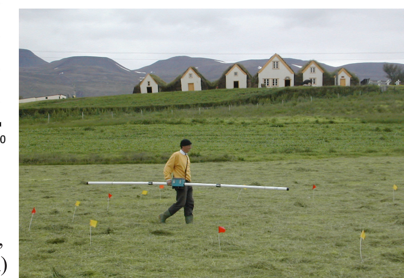
Figure 5. Using the EM-31 at Glaumbær. The turf walls directly below the operator are preserved 60 cm high.
